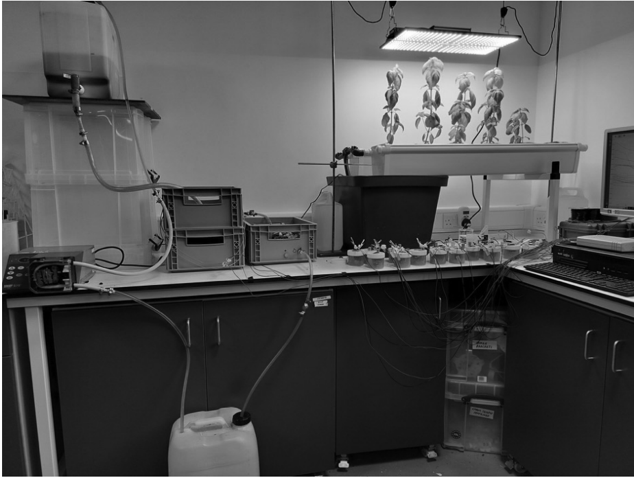
Figure 6. Microbial Hydroponics, integration of hydroponics and MFCs, University of Southampton, UK. Photograph courtesy the Microbial Hydroponics consortium, taken by Dibyojoty Nath, 2024.
